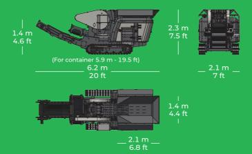
Recycling on site demolition and construction waste is a cost-efficient method of avoiding large landfill costs, onsite recycling and reducing demolition rubble to a useable product. The K-JC 604, a 600x400mm jaw crusher fitted with an integrated vibrating feeder, the material to be processed is moved in a fast, constant linear action into the jaw. The CSS is adjusted hydraulically by remote control.
